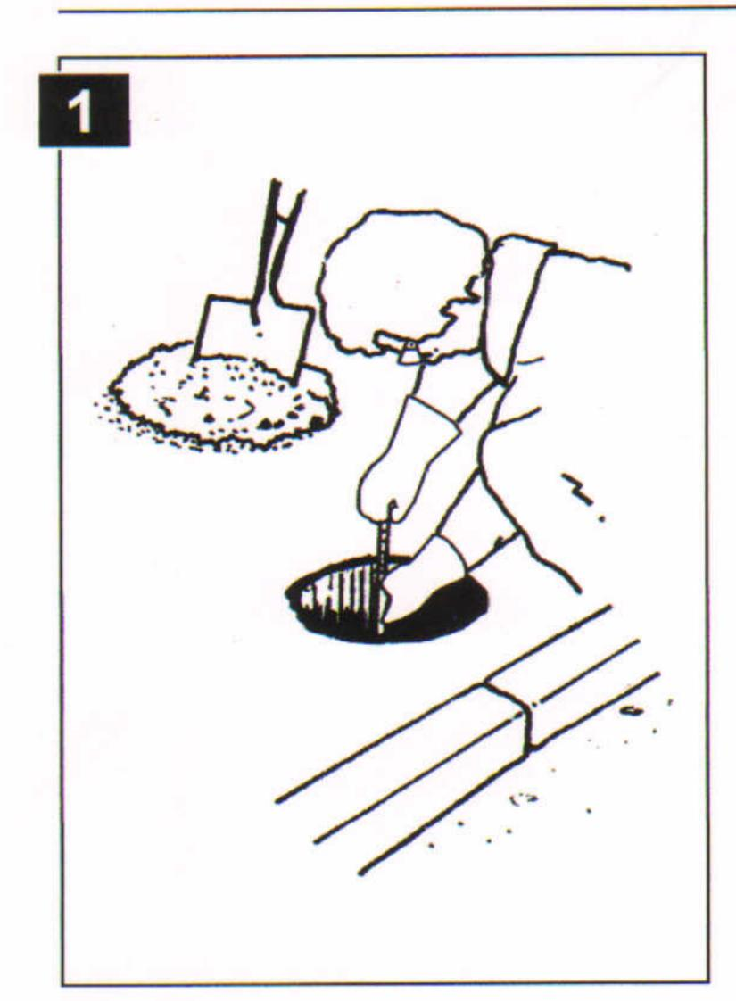
1 Mark up and dig hole approximately 330mm in diameter x 530mm deep minimum.
